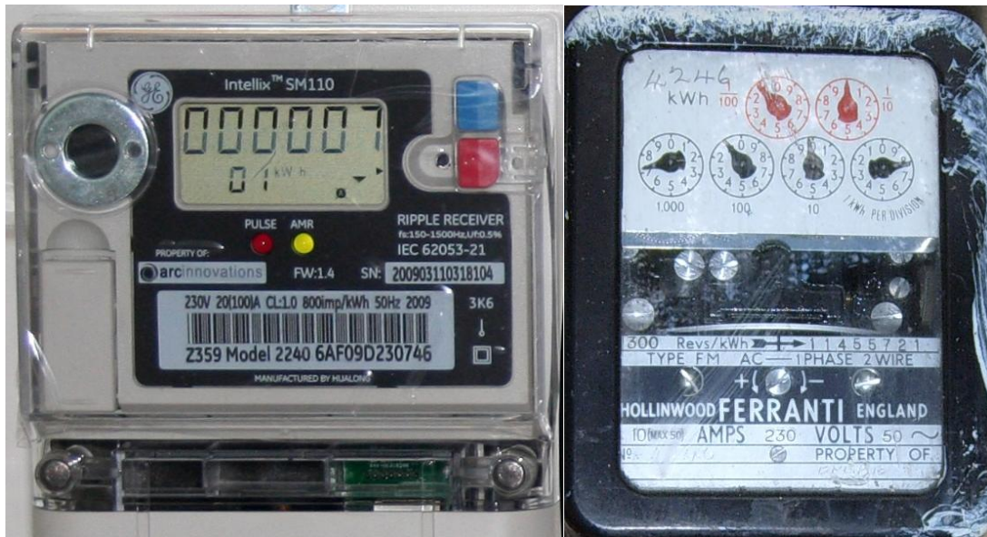
Figure 1. A typical Smart Meter and a traditional electromechanical meter
